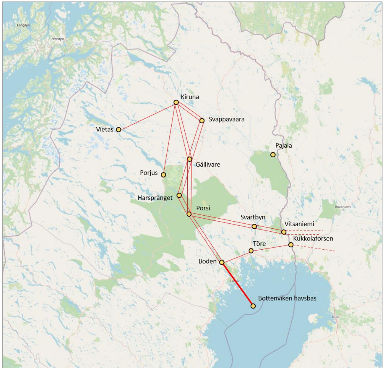
Figure 15. Stage 2 in the power transmission scenario will provide an additional capacity of 2.8 MW summarizing to total capacity of 6.6 GW to Kiruna with redundant supply routes. The additional power is assumed to transfer a significant quantity of Finnish wind power.
