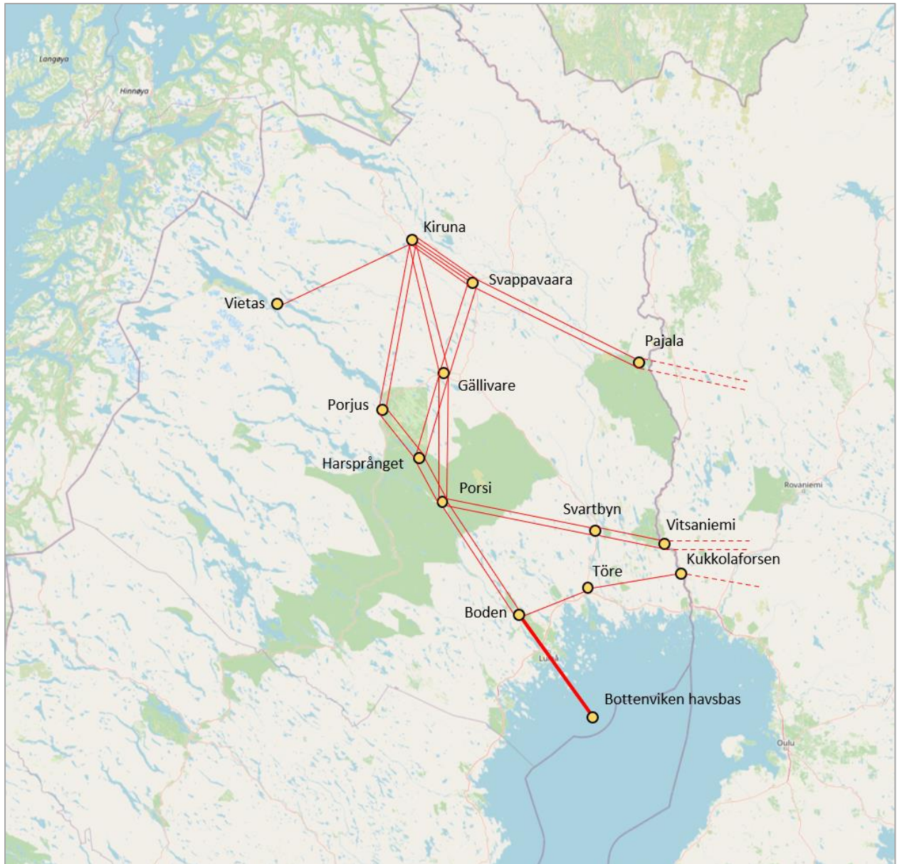
Figure 16. Stage 3 in the power transmission scenario will provide an additional capacity of 4.2 MW summarizing to total capacity of 10.8 GW to Kiruna with redundant supply routes. The additional power is assumed to transfer a significant quantity of Finnish wind power in the very north, through Pajala.
