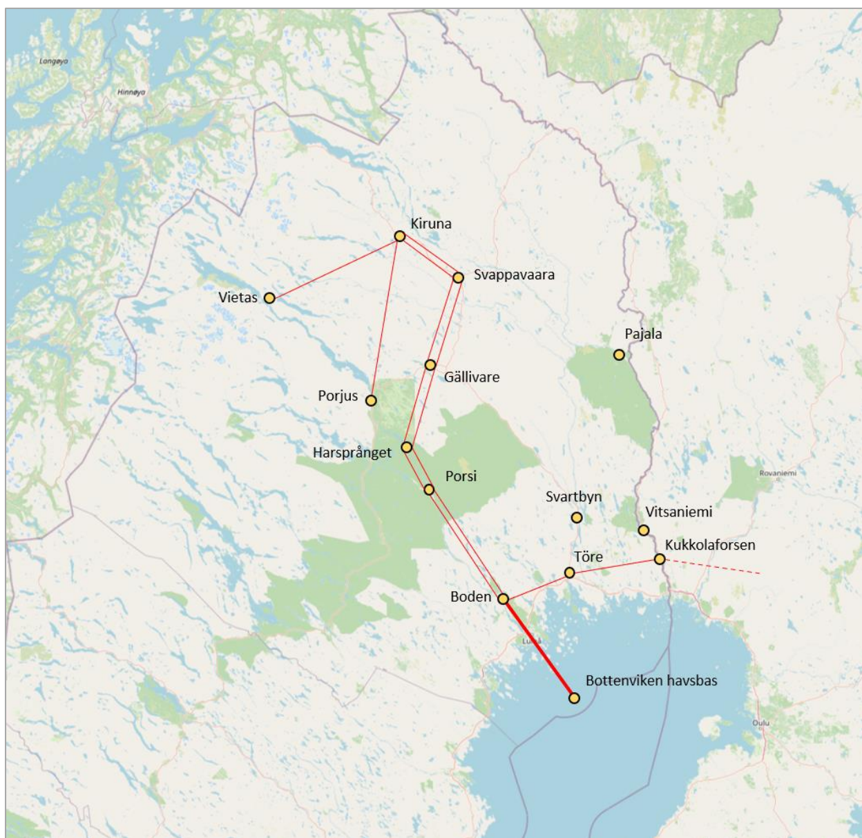
Figure 14. Stage 1 in the power transmission scenario will provide a capacity of 3.8 GW to Kiruna with redundant supply routes. The offshore wind in the Bothnian Bay will have a capacity of 1.4 GW.
